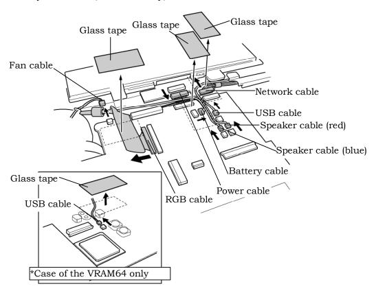
Figure 4-26 Removing the system board (1)
